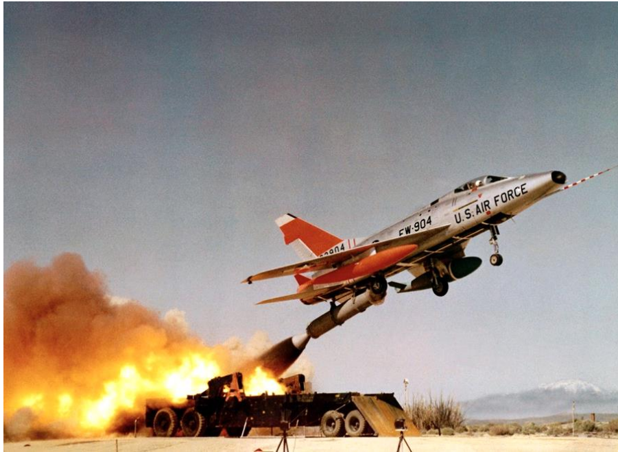
F-100 fighter in a zero length launch
